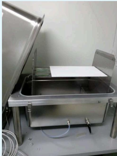
**Photo of open chamber with specimen and glass slide containing the formaldehyde requiring abatement**
